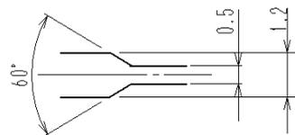
Unless otherwise specified, tolerance:  $\pm 0.1\text{mm}$
