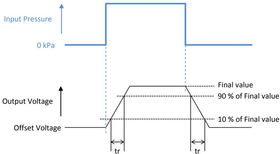
\*10) Output voltage (Vout) is sampled and held by the internal sampling / hold block. Sampling frequency (fs) is 1 kHz. The output voltage is changed stepwise every approximately 1millisecond.
