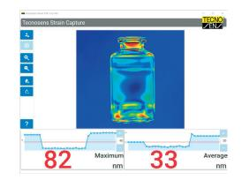
Measure annealing stress in order to avoid unwanted fragility of the container glass.
