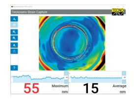
Strain Capture can measure annealing stress on the bottom of the bottle, rejecting automatically pieces that are out of the required tolerance.
