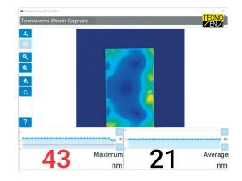
Strain Capture allows to measure the stress distribution on flat glass. The distribution must be even so to avoid optical distortions and glass fragility
