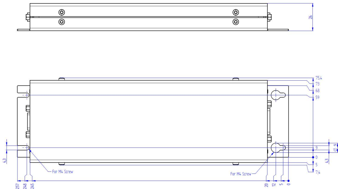
Figure 5: View of the electronics housing. Dimensions in mm
