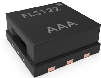
6-pin DFN package 3.5 mm × 3.5 mm footprint 2 mm overall height
