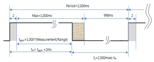
EX) t<sub>H</sub> (High Pulse Width) calculation for 50% LEL in 100% LEL Range.
