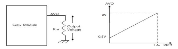
Measured Voltage 0.5V~4.5V match proportionally to 0 ~ 5,000ppm.
