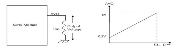
Measured Voltage 0.5V~4.5V match proportionally to 0  $\sim$  5,000ppm.
