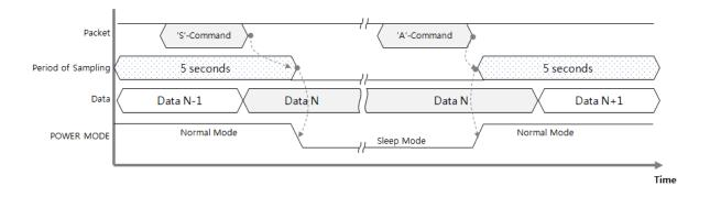
To go into the Sleep mode, Master should send Command packet to Sensor's RX-line and should be kept to 'High' until Master send the Wake-up Command to finish Sleep mode.
