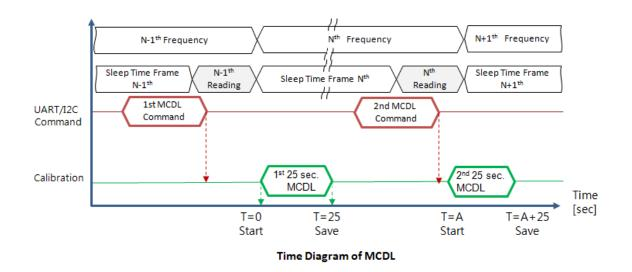
Method 1. UART Command Set; pin-3 (UART-RX) and pin-5 (UART-TX) to Main-Board. (J2-13pin and J2-14pin are available for BtoB connector User as well)
