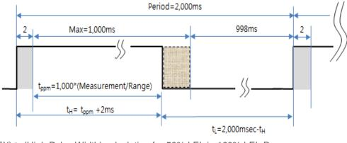
EX) t<sub>H</sub> (High Pulse Width) calculation for 50% LEL in 100% LEL Range. \*Measurement(% LEL) = 50% LEL =  $(t_H-2m_s)/2,000m_{sec} \times Range(% LEL)$ , \*t<sub>H</sub>= 1,000 msec \* (50% LEL / 100% LEL) + 2msec = 502msec (cf:  $T_L$  = Period -  $t_{H=}$  2,000 msec - 502 msec = 1,498 msec.)
