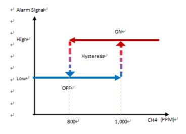
EK-100SL series is available for customer to enable to change alarm activation & deactivation point. **PWM Descriptions : Option**
