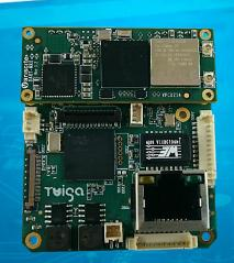
Red Mamba IP video encoding board has been specifically designed for compact embedded vision systems.
