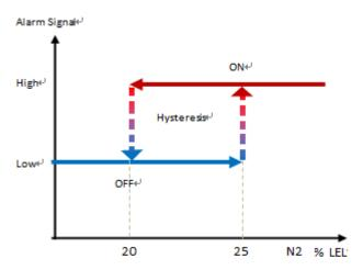
EK-100SL series is available for customer to enable to change alarm activation & deactivation point.
