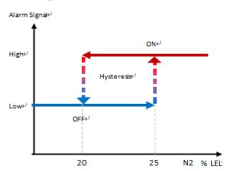
2<sup>nd</sup> Alarm use VoL / Voн TTL signal Switching instead of SPST (Single Pole Single Throw) method. EK-100SL series is available for customer to enable to change alarm activation & deactivation point.
