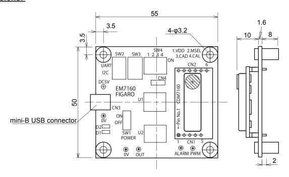
Note 1) Standard CDM7160 CO2 sensor modules (without terminal pins) are available for additional purchase. To attach a standard CDM7160 to the evaluation module, terminal pins available in the marketplace should be soldered to the standard CDM7160.
