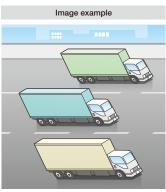
A "Rolling Shutter CMOS Sensor," as employed in general camera modules, captures target images sequentially from upper to lower scan-lines; artifacts are incurred on fast moving objects (focal plane distortion) due to the sequential delay to run each scan.
