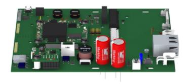
With the new LadonBoard, designed and developed by Tecnosens, you can now manage several video signals of various kinds at the same time: from the IP stream of regular Onvif cameras, up to the uncompressed streaming of high-resolution sensors.
