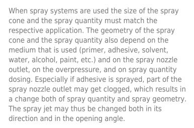
A spray jet control system in time informs the user about such a change of the spray jet.
