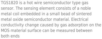
of the noble metal coil as a change in the combined resistance of the MOS material and the noble metal coil.
