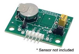
This module is useful for evaluating basic performances of TGS5141 gas sensor and as a reference of application circuit.
