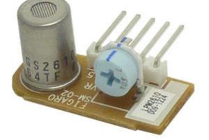
The LPM2610 is a pre-calibrated module for LP gas alarms which is precisely calibrated in Figaro's humidity and temperature controlled facility. The module uses TGS2610-C00.
