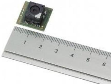
Sony is expanding its popular FCB Block Camera Series with the introduction of an ultra-compact, all-in-one color camera - the FCB-MA130 - which supports both moving pictures and still images.
