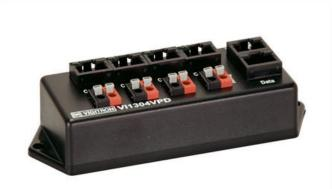
Combines video, power and data into a single RJ-45 4-pair cable, support up to four cameras with power indicator for each camera.
