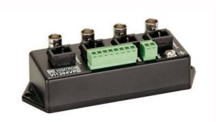
The Vi1204VPD is a passive transceiver device that combines video, PTZ data and camera power over a single 4-pair UTP cable to simplify CCTV installations in a structured wiring environment. It supports up to 4 cameras for up to 750 ft. (228 m) and is designed to be installed in the control room. The Vi1204VPD receives low-voltage camera power from any third party multi output Class II power supply. Each camera power output is equipped with a self-resetting fuse for extra protection.
